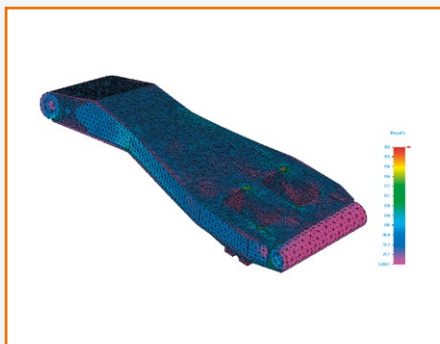
Strength calculation by means of the finite element method.
